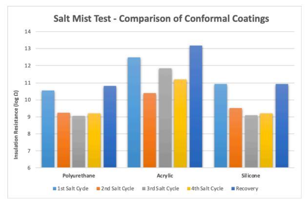
Graph 1 – Comparison of conformal coating performance in a salt mist environment
