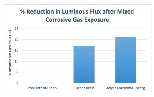
Graph 4 – Change in luminous flux after exposure to mixed corrosive gas
